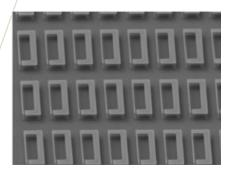
Dense array of identical THz resonators © Erganeo
