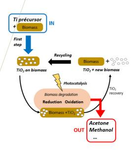
Biomass conversion - Biogas and biofuels production Photocatalysis - Energy production
