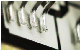
Degradations: detachment of connection wires
