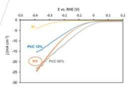
Current-voltage curve measured at 10 mV/s in 0.1 M KOH
